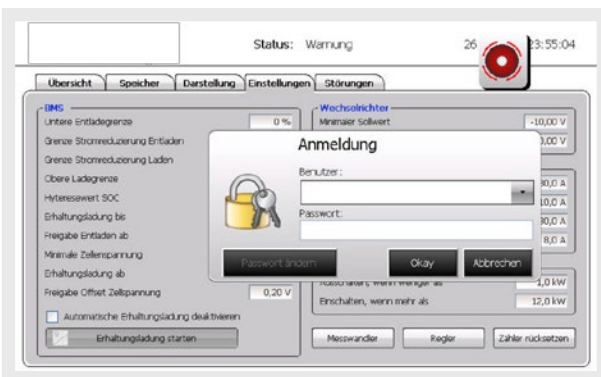
Page showing that an alarm has been triggered, and the HMI is prompting for user authentication before menu access is granted.
