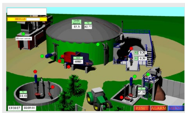
Top-level menu for a biogas facility in Italy. Submenus, system reset, and alarm are all accessible from this page.
