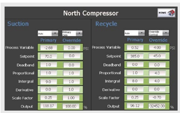
Controls for the North Compressor.
