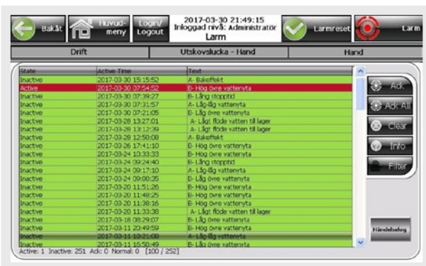
The alarms page displays messages from subsystems. These messages can be investigated, acknowledged, cleared, and/or filtered.
