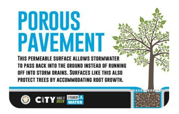
The <u>porous pavement</u> allows rain to enter the ground instead of flowing into sewers. This is part of the smart green infrastructure plan to manage stormwater runoff while also providing a safe and accessible route for all users.
